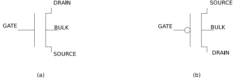
Figure 2: MOS transistor schematic symbols used in the thesis (a) NMOS (b) PMOS
